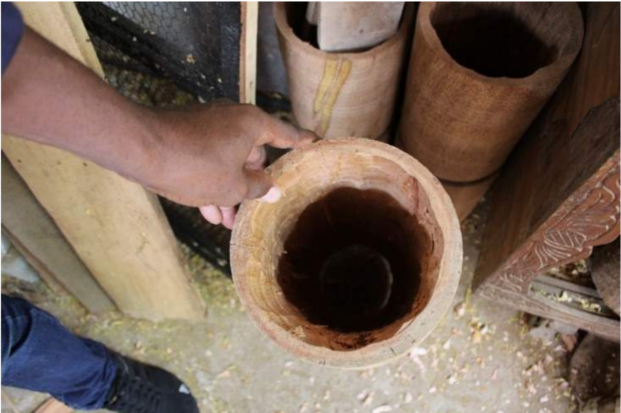
Figure 1: A hollowed-out drum body. Produced with traditional iron tools. Photography by Geethika Abeysekara, 1 st April, 2023, Kurugama, Kandy, Sri Lanka.
