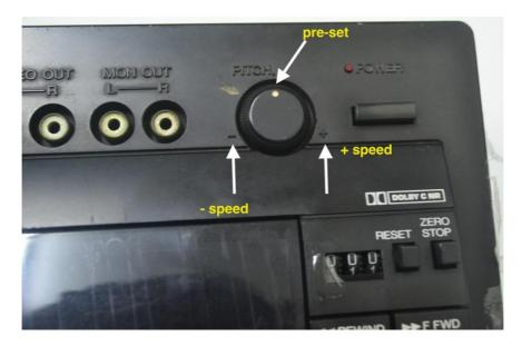
FIGURE 7: Tape speed of the replay unit.
