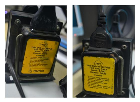
FIGURE 11a and b: Transformer from 220 volts to 115 volts.
