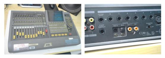
FIGURE 4: The front panel and its controller; Figure 5 the rear are the sockets for other possible connections (Photographs and all following photographs of the author).
