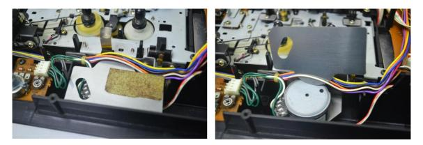
FIGURE 16: A protector of magnetic fields derived from the single DC servo motor 3 3/4ips - twice the normal cassette speed.
