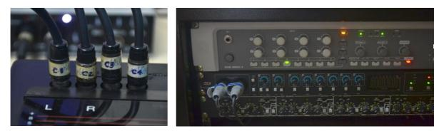
FIGURE 23a and b: Direct RCA outputs - 10dBv to the inputs of audio interface independently.
