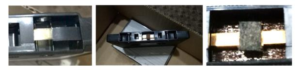
FIGURE 8: Deterioration due to fungus; FIGURE 9a and b: Mechanical issue such as broken tapes, rusted magnetic shield.
