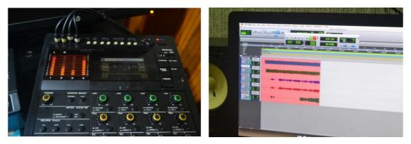
FIGURE 24a and b: Migration of audio signal (real-time) from the replay unit of independent outputs to the direct inputs of the Digital Audio Workstation with the bit resolution and sampling rate recommended by the IASA-TC04.
