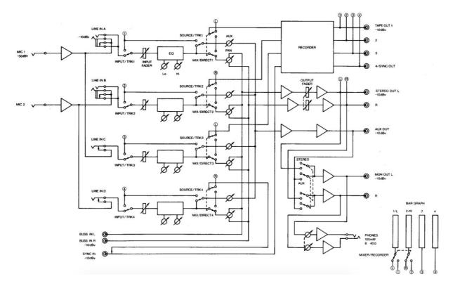
FIGURE 3: Block diagram of the FOSTEX 160 Multitracker Recorder/Mixer, a representation of the input and the output sections of the device.
