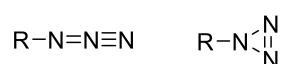
Figure 1: Postulated structures of azides. The linear structure was suggested by THIELE (left), and the cyclic structure was proposed by CURTIUS and HANTZSCH (right).
